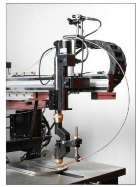
This system was assembled using standard Weldlogic products to provide an automatic Plasma, keyhole/Plasma Arc welding system.
