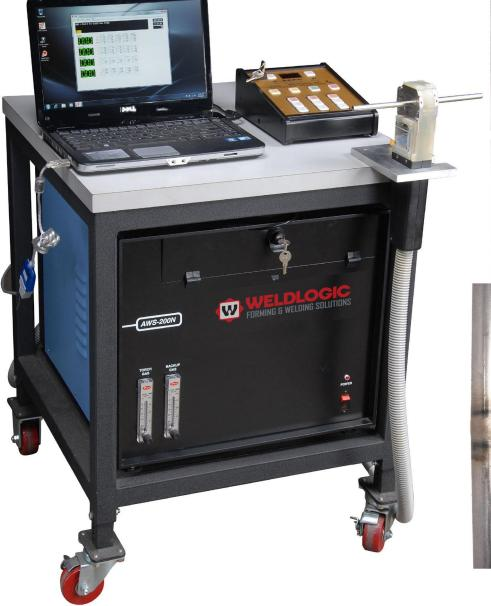
Weldlogic Inc. combined 2 of our standard products, the AWS-200 Advanced Welding System and a Orbital Weld Head. This combination enables a high reliability thermacouple manufacture the capability to produce X-ray clear tube to tube splices.
