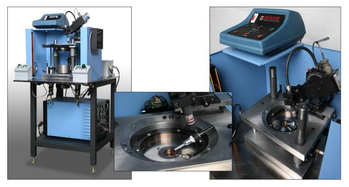
Weldlogic's I.D. bellows station provides a welding cell to join bellows as thin as .002" thick. The precision die set fixture design provides precision alignment of the bellow assemblies providing extremely uniform weld results.
