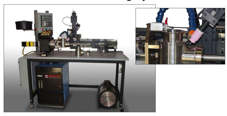
This AWS-300 / 6100 C.N.C. Welding System was manufactured to provide a Circumferential Welding System to easily and precisely produce complex 2 axis Saddle welds on High Purity Valve Assemblies. The valves required complex motion profiles to welds both the I.D. and O.D. saddle weld joints with wire feed.
