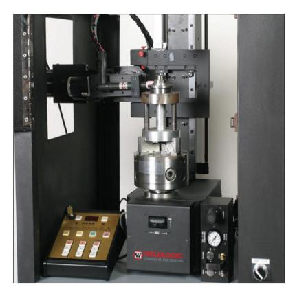
This AWS-150/6100 System was configured to provide a verticle production welding work cell.
