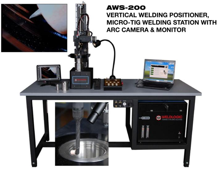
This AWS-200 "Micro-Tig" welding system was designed by Weldlogic engineers to produce a low current I.D. weld on a high reliability flange to tube assembly. The I.D. weld was located in a recessed area that made it impossible to align the welding electrode reliably over the weld joint. Special tooling was developed to accomidate the full range of diameters and part lengths.
