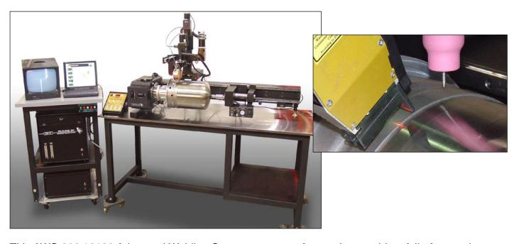
This AWS-300 / 6100 Advanced Welding System was manufactured to provide a fully Automatic Circumferential welding cell. The part purge time and multipass weld time could run up to 10 minutes per part. The customer required minimal labor content and 100% yield.
