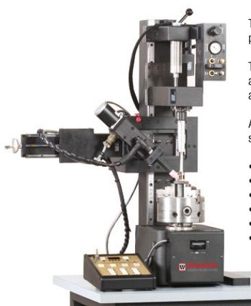
The PWL Vertical 6100 Welding System was configured to provide a verticle production welding work cell.
