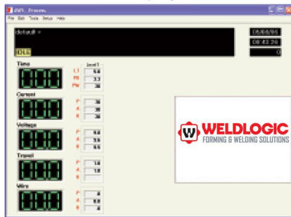
Program up to 9 levels per weld schedule plus level sloping
