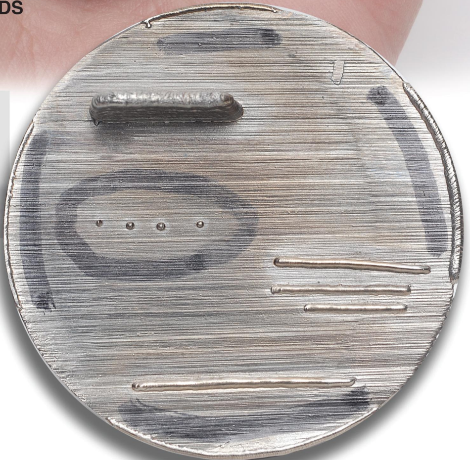
Tool Steel Scrap Used to test the Weldlogic Microscopic Weld Station
