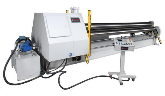
A DC hydraulic directional control valve is used on each axis. The position of each axis is sent back to the PLC by optical encoders to ensure accurate positioning. In addition to the three axis the PLC also features digital input and output forcontrolling the hydraulic drop-arm and the manual mode control functions.
