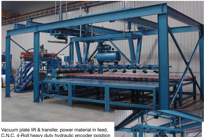
Vacuum plate lift & transfer, power material in feed, C.N.C. 4-Roll heavy duty hydraulic encoder position based roll forming with overhead tank support, tank ejector with Transfer to Seam Welder.
