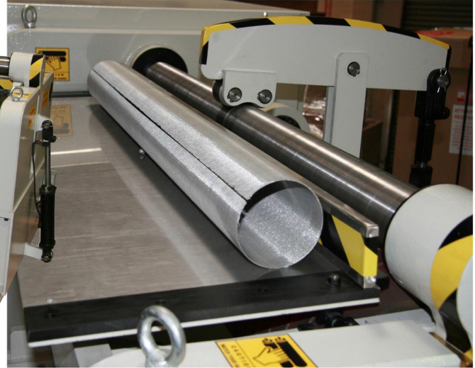
The roller has a removable deflection beam to enable smaller diameters in shorter lengths
