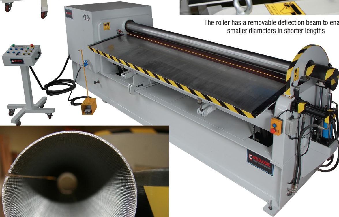
10 foot custom built urethane roller to manufacture down hole specialty filters for the oil and gas industries
