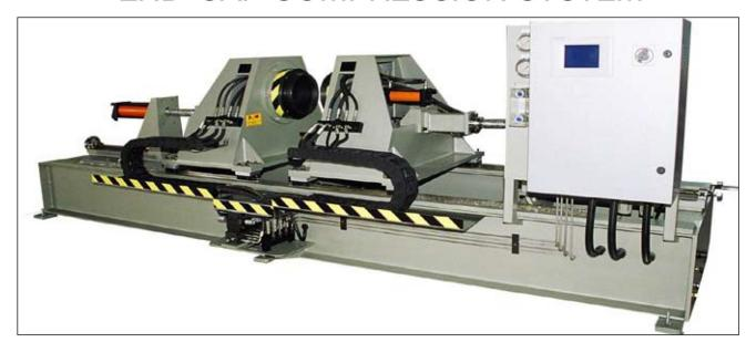
This specially designed machine was developed to serve the tank manufacturing industry. The system is designed to cradle, lift and center the bell ended tank assembly in various diameters and length based on the specific product line range.
