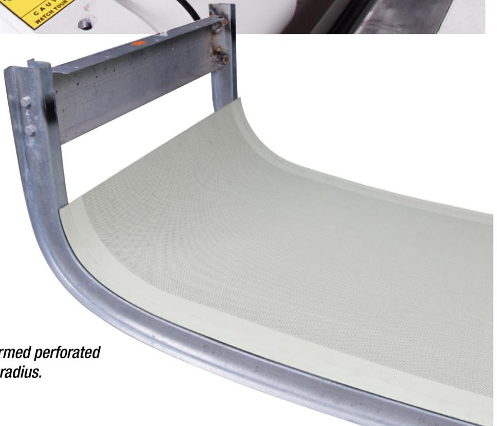
*Bus ceiling panel with formed perforated panel with smooth fitted radius.*
