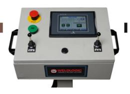
series PLC configured for closed loop position control via AC servo motors for the material feed and forming operations. The control system is very flexible in programming to form many variations of round and non-round parts. The operator interface is a Touch Screen HMI. The touch screen is capable of storing over 100 part programs of up to 50 forming steps per programs.
