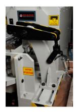
**DROP ARM:** Removal of the finished cylinder is accomplished at the operator's pendant by push button. The drop arm is moved open and closed by a pneumatic cylinder that is locked in place with a pilot operated check valve.
