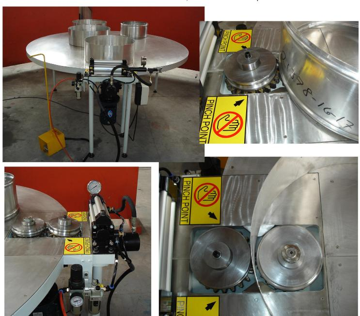
This machine was specifically designed to accommodate tube beading from 6" - 65" in materials up to .125" thick.
