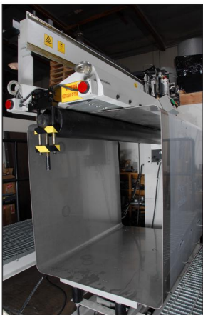
Hydraulically Controlled Transfer Cart transports 500-lbs tanks from forming system to elevated seam welder.
