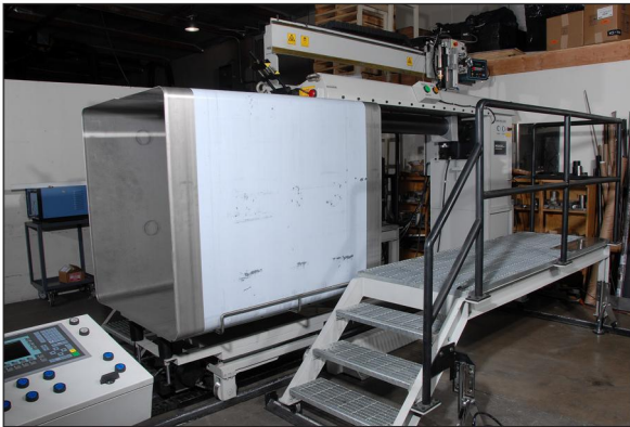
Hydraulically Controlled Transfer Cart transports 500-lbs tanks from forming system to elevated seam welder.
