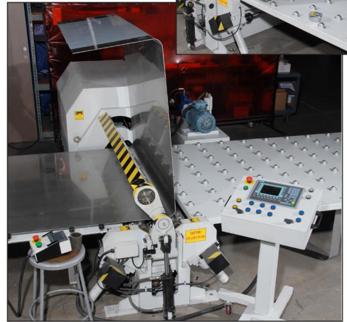
5 Axis C.N.C. Specialized Roll Forming System performs complex forming program to produce a 2" radius square tank in 2-ft / 6-ft squares.
