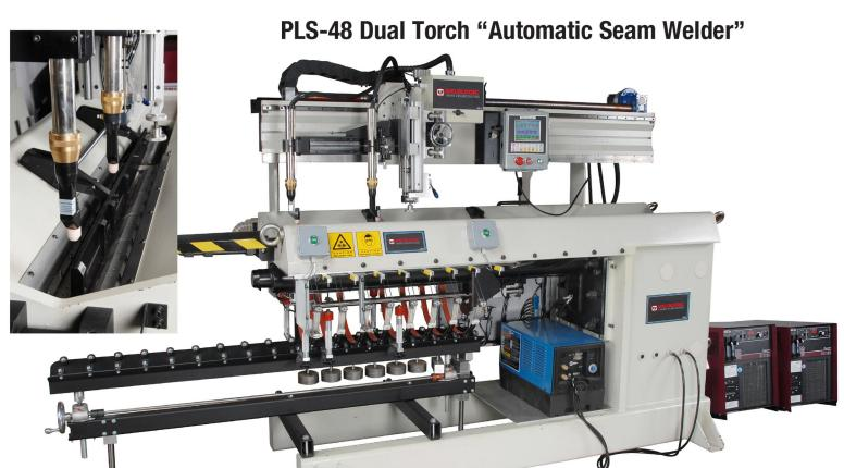
Weldlogic Engineering were tasked to design and manufacture a high production dual plasma torch seam welder to enable a low skilled operator to run both our automatic roller and automatic seam welder.
