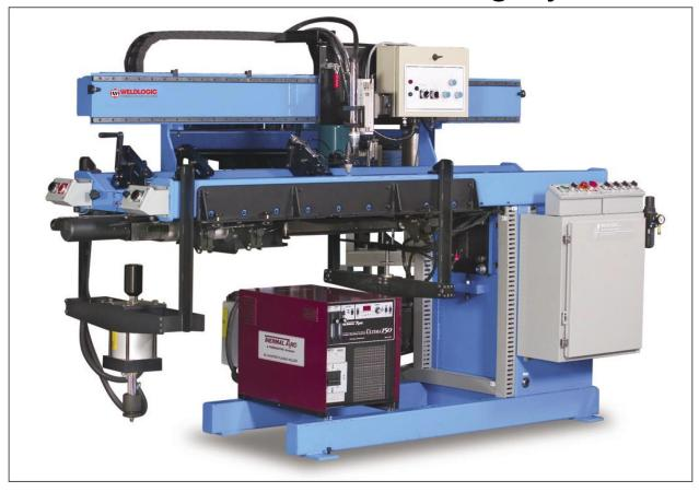
The PLS-60 Precision Longitudinal Seam Welder uses automatic material handling and fixturing mechanisms to produce high quality Automatic Seam Welds with TIG, Plasma, MIG or Laser at production rates of 90 -120 parts per hour.
