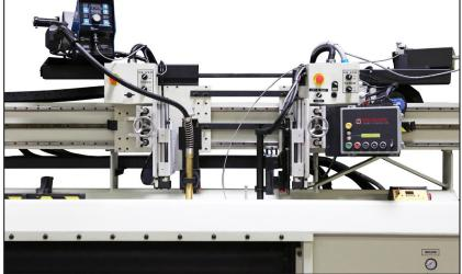
**Weldlogic PLS Weld Seamers** are designed for straight line welding of all weldable metals in thicknesses from .005" to 1/2" and lengths up to 15 feet.
