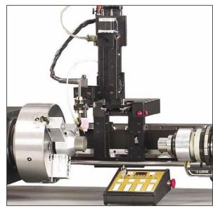
This AWS-150/300-6100 system required a mechanical engineered solution to enable the lathe spindle to pass thru a 3.8" diameter titanium tube and weld it to a end cap assembly.
