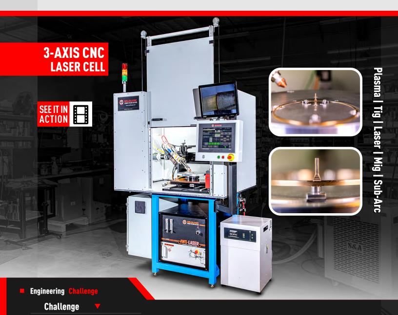
■ Build an ultra-precision 3-axis weld cell that enables high accuracy positioning and high accuracy delivery of the correct laser energy based on the position of the Beryllium component.
