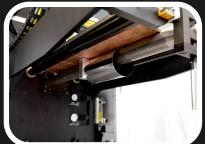
Weldlogic process specialist chose laser welding and our UPS-24 Ultra Precision Seam Welder to achieve CNC quality laser welds in conjuntion with a seam tracker and vision system for live inspection during welding.
