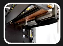
Weldlogic process specialist chose laser welding and our UPS-24 Ultra Precision Seam Welder to achieve CNC quality laser welds in conjuntion with a seam tracker and vision system for live inspection during welding.
