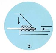
Clamp sheet in position extract positioning block
